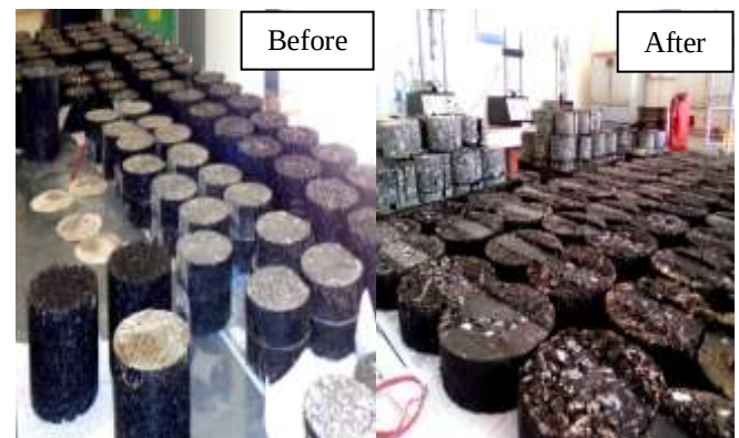
Fig. 10. Gyratory Samples Before and After Tests
