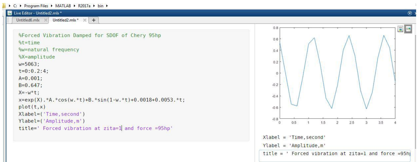
Figure 10 Forced vibration of the system at 95hp and 1 damping factor
