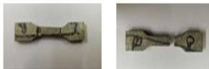
Figure 12 AMC MS-150 specimens-Before and after tensile test
