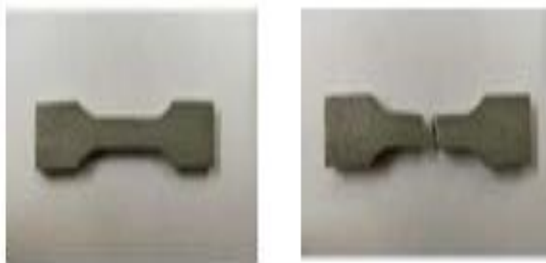
Figure 11 Base alloy specimens-Before and after tensile test
