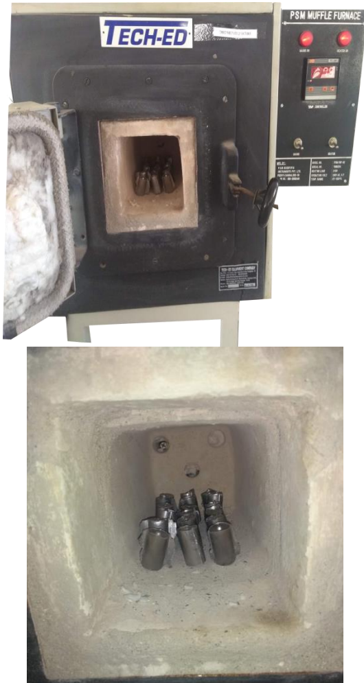
Fig3. Muffle furnace and Sintering of specimens
