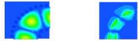
Fig.3 Distribution of the E-field along SIW and microstrip bends
