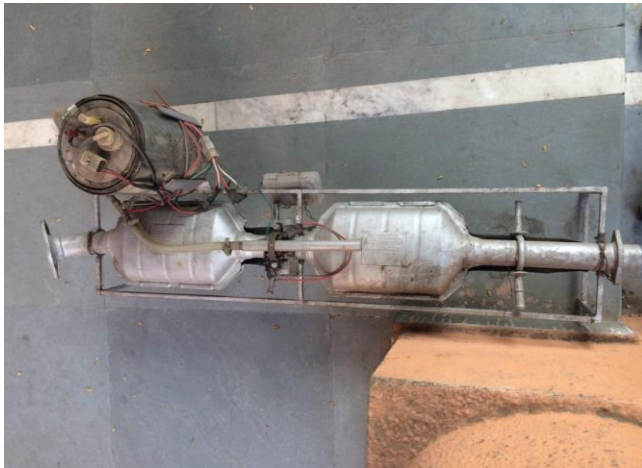
Figure 5: Modified SCR System
