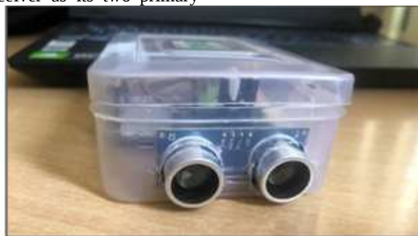
Fig. 3 Device containing Ultrasonic Sensor
