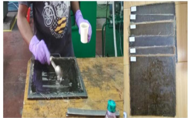
Fig. 3. Hand layup of composites
