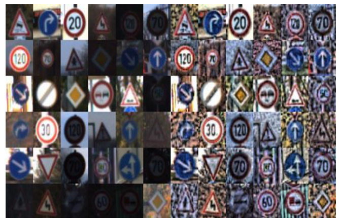
Fig. 1. Original Images are present on the left side. After applying CLAHE, image contrast is improved and the images are seen on the right side
