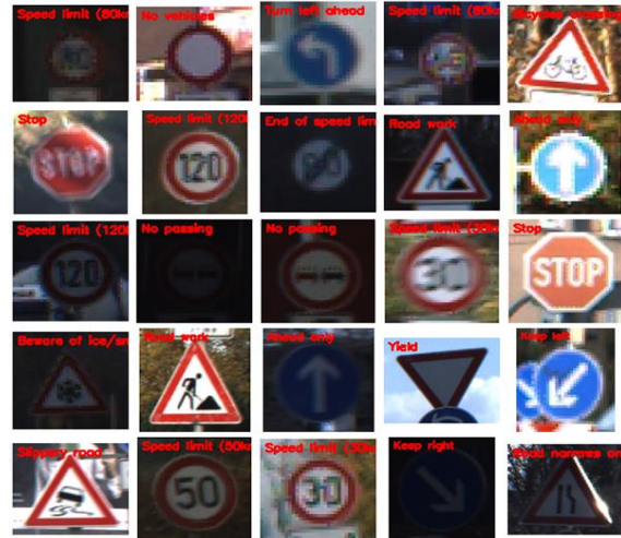
Fig. 5. Result of Traffic Sign Recognition and Classification
