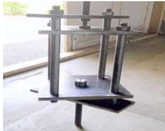
Figure 3.5 Small punch test fixture with specimen holder, punch holder, punch & connecting rods in an assembled mode.
