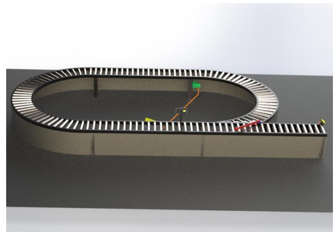
Fig. 4. Image of the belt driven roller conveyor
