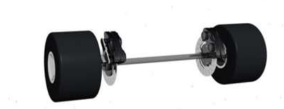
Fig. 13: Disk Brake Arrangement
