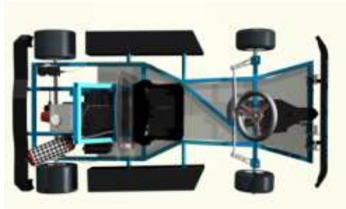
Figure 3: Top View of CAD Model of Go- Kart
