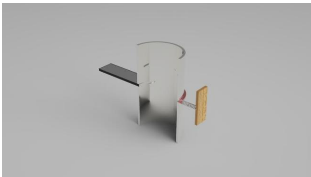
Fig 6. The mechanism used for glass/colour filter introduction
