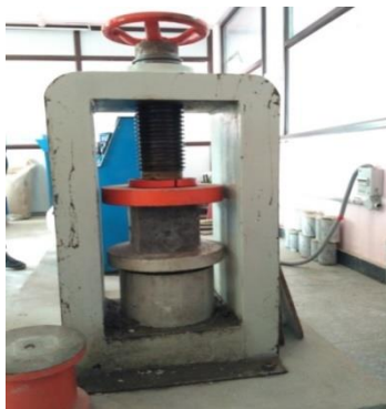
Fig-1: testing of cube specimen
