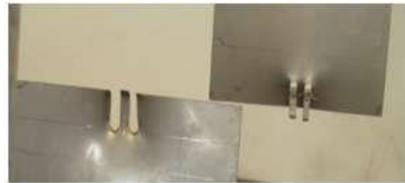
Fig.5 .Pull out failure mode
