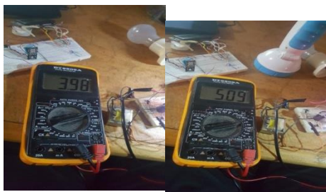
Fig. 19. Rectified LM317 Input and output Voltage (Breadboard)
