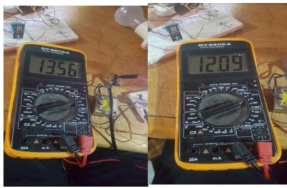
Fig. 16. Rectified LM7812 Input and output Voltage (Breadboard)
