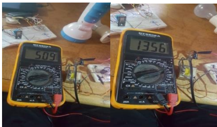
Fig. 17. Rectified LM7805 Input and output Voltage (Breadboard)
