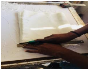
Fig 8: Cutting of glass fiber
