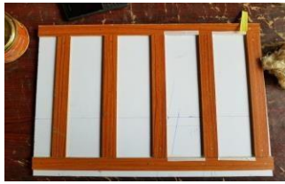
Fig 7: wooden mold to prepare composite material
