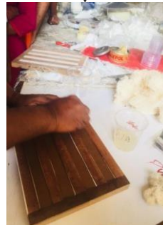
Fig 10: applying PVA coating on mold
