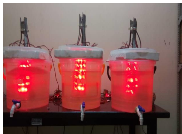
Fig. 1 Modified Stirred-Tank Photobioreactors MSTPBRs set-up
