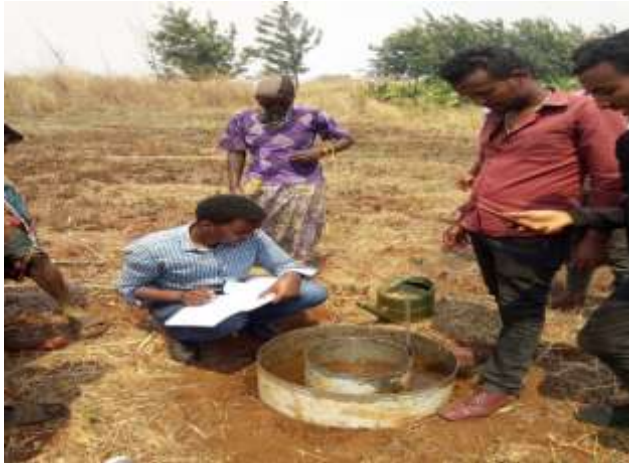
Figure2.3: Infiltration rate determination Golda small scale irrigation scheme
