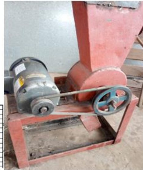
Figure 4: Exploded view of a modified palm nuts cracker Figure 5: The developed centrifugal palm nuts cracker
