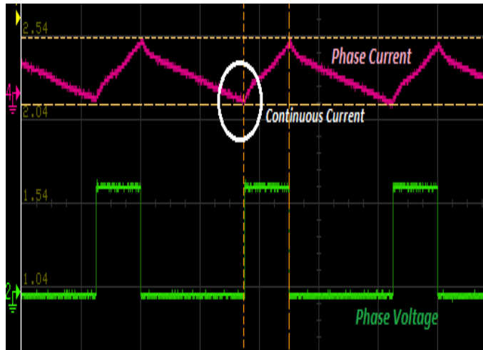
Fig. 5. Phase voltage and current of motor with bus clamped PWM technique
