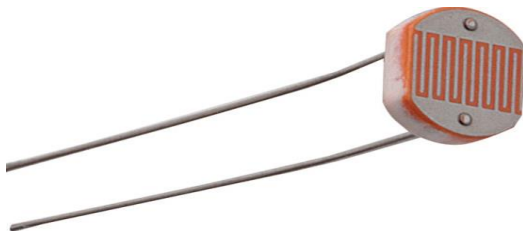
2. The second way is to use a simple laser where it will be aimed on a photoresistor located on the other side of the conveyor belt just opposite of the laser. In this case, our sensor will be the photoresistor where it will be placed in a black frame to have as little interference as possible from the outside light. So when the light beam of the laser is cut off from the bottle, the photoresistor will change value and as a result the process starts and the camera is switched on.
