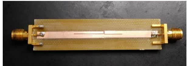
Figure 9. Prototype Circuit for Dual band stop filters at 3.25 and 5.5 GHz
