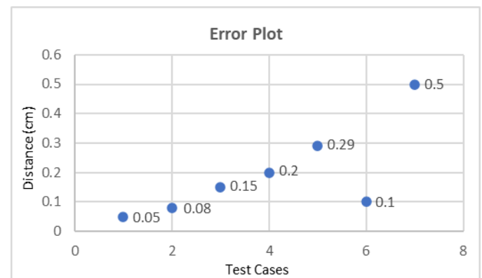
Fig. 10. Error Points of Ultrasonic Sensor
