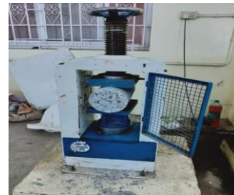
Fig 6 – Split tensile test
