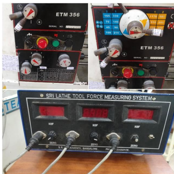
Figure 2: Lathe Machine And Machine-Tool Dynamometer
