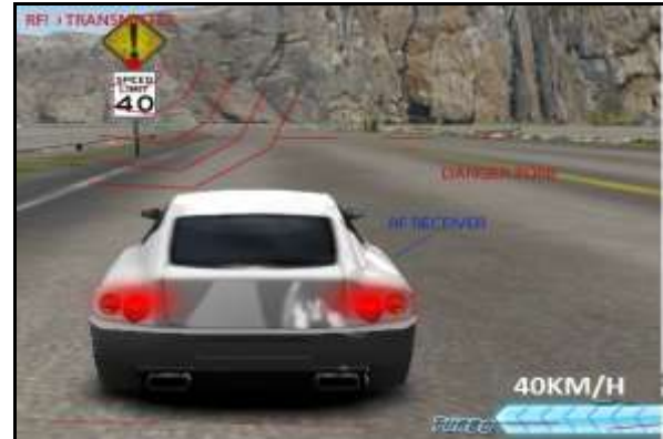
Fig. 1. RF transmitter/receiver antenna on signboard and vehicle respectively.
