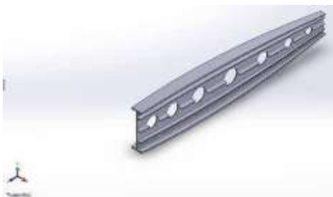
Figure 4.1 Modeling of rib structure with circular holes
