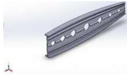
Figure 4.2 Modeling of rib structure with circular holes
