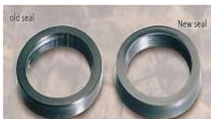
Figure 21 the Contamination Damage in Rod Seal
