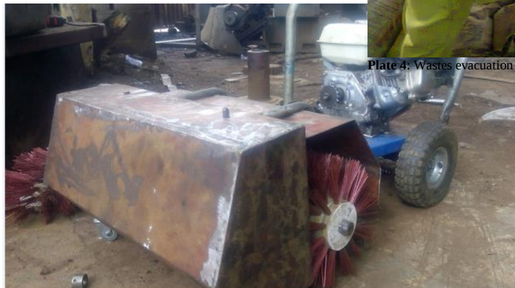
Plate 2: The fabricated portable sweeping machine
