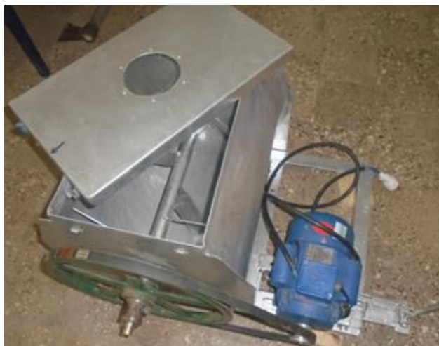
Fig. 2 Electric motor operated milk churner
