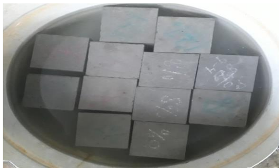
Fig. 5 Curing of specimens
