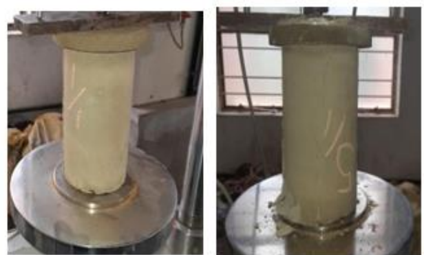
Fig.5.4: Failure Pattern of Fly Ash Based Material Specimen
