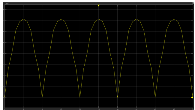
Figure 22: Flow coefficient versus Time at P_{max} set to 5000
