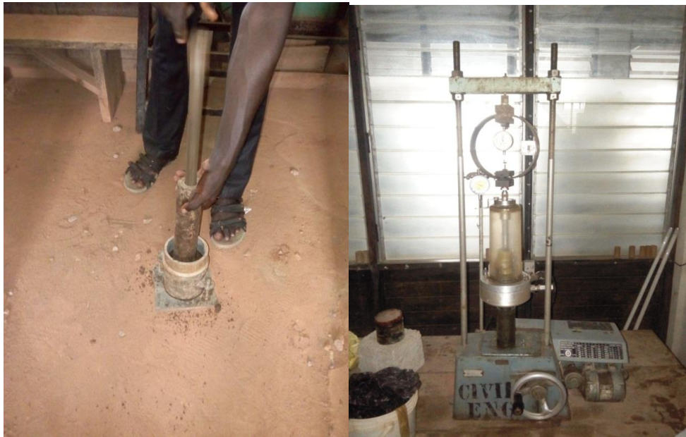
Fig 1: Experimental operation (Compaction and Tri-axial Test)
