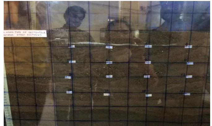
Fig 1. Geometry of the planar geotextile-reinforced foundation bed.
