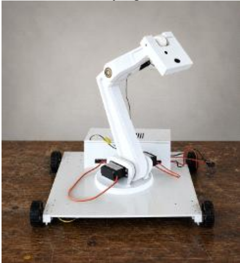
Fig. 1.SUNIL rover with mounted ESP32-CAM and robotic arm.
