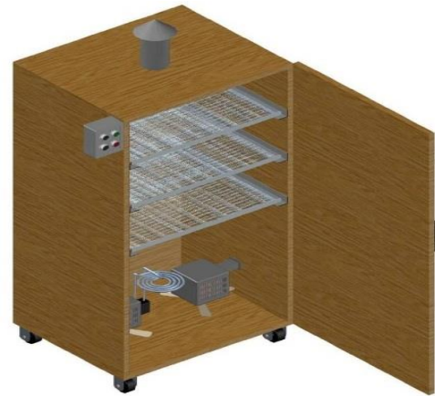
Figure 1 a. Assembled drawing of the vegetable dryer
