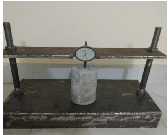
Fig. 1. Length comparator with tested material.
