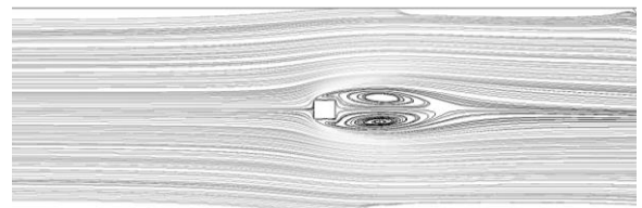
Figure 18: Time-mean streamlines for square cylinder at \alpha = 90^\circ
