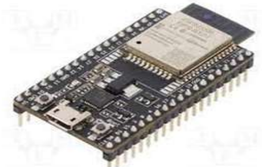
Fig. 2. ESP 32 - Microcontroller and Wifi
