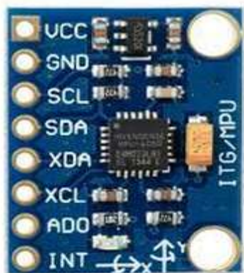
Fig. 3. MPU6050 - Gyroscope and Accelerometer
