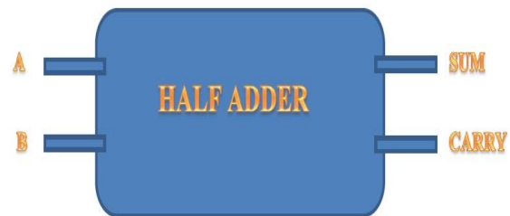
Fig.1 Block diagram for half adder
