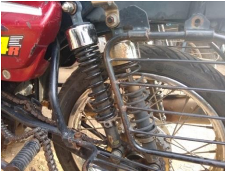
Fig. 1. Existing rear suspension system in TVS Max 100 R model
