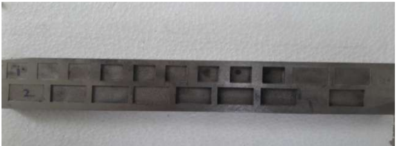
Fig 3.4 Inconel600 work piece after machining with Copper and Graphite Tool
