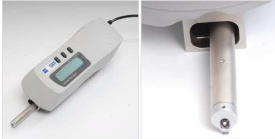
Figure 3.1 Measuring surface roughness by using HANDYSURF
