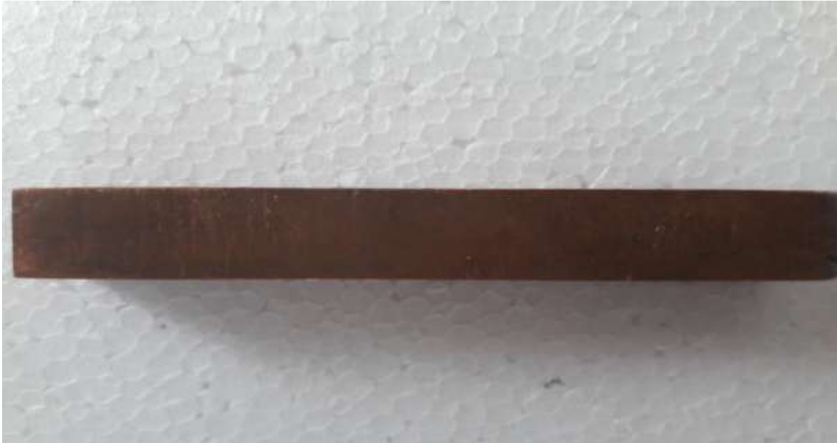
Fig 3.3 copper tool after machining inconel600 workpiece
