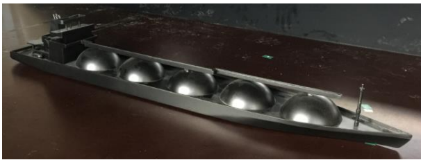
Fig. 4. Real ship model with sphere tank for doing wind tunnel test
