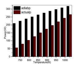
Fig. 9 Relationship between hot source temperature and engine power
