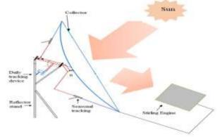
Fig. 1 Schematic diagram of solar parabolic dish system
