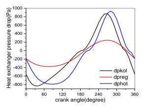
Fig. 17 Heat exchanger pressure drops virus crank angle
