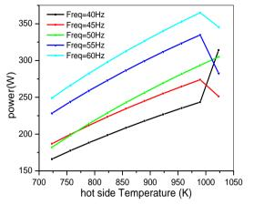
Fig. 8 Relationship between hot source temperature and engine power
