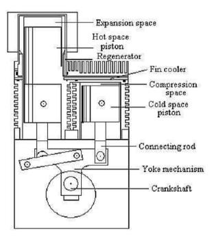
Fig. 2 gamma Stirling engine
