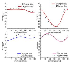
Fig. 12 Heat transferred within the different cells
