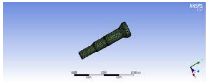
Fig. 3. Meshing of Punch Model Modified (3)
