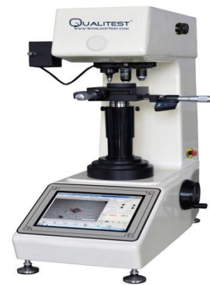
Fig 3Vikers hardness testing machine
