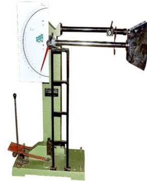
Fig 2 Impact testing machine
