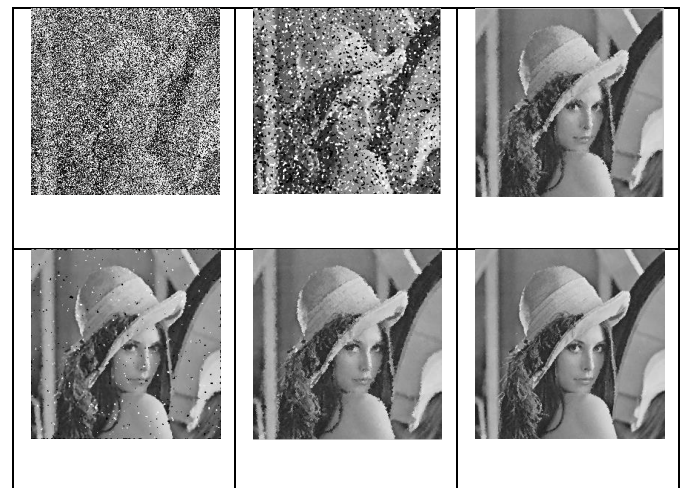
Fig. 2 (a) image contaminated with 60% density of salt-and-pepper noise. Results obtained using (b) SMF (c) ADMF (d) MDBUTMF (e) HPDF (f) Detail Preserving Filter
