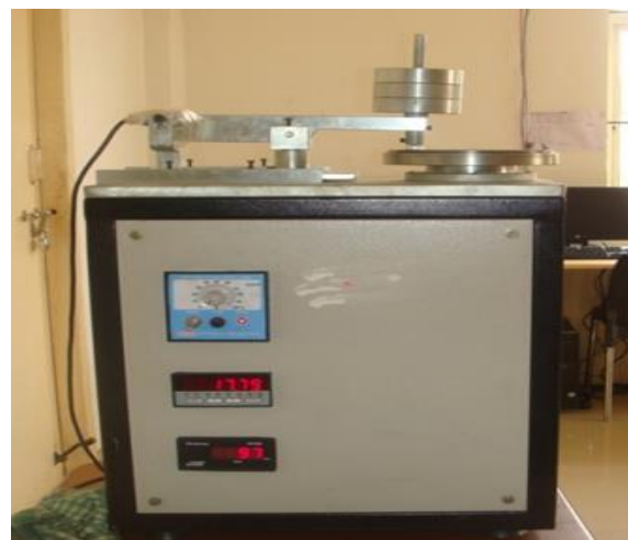
Fig. 7 testing machine for pin wear
